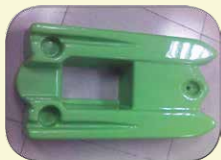
遥控船 1.5mm Clear PETG sheet with spray color 400mm x 600mm
